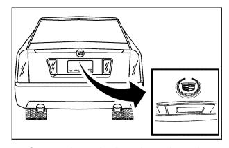
Squeeze the trunk release button located on the rear of the trunk lid above the license plate, as long as you have your keyless access transmitter with you. Entry occurs when the button is being pressed and the vehicle recognizes the transmitter. The vehicle must be in PARK (P) and the valet mode turned off.
